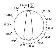
When the time that has been programmed has lapsed, the buzzer sounds and at the same time the oven is automatically switched off. To use the oven with the manual function, excluding the timer, put the knob back to its original position, rotating it in an anticlockwise direction by one notch until the reference of the knob coincides with the by symbol on the control panel.
