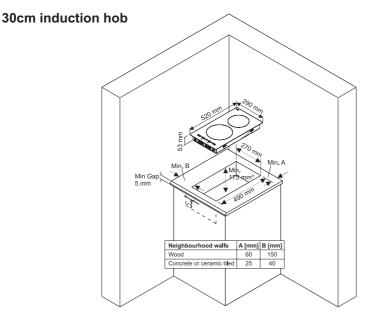
\*: In the case of installation over built in oven, distance should be min. 10 mm.
