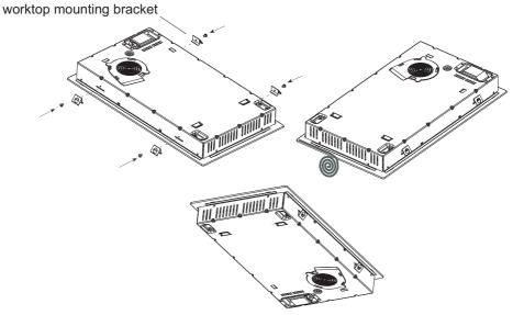
$\cdot$  Secure the hob in place by putting it into cutout on the work surface.
