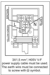
For the induction hob, the cable must be H05VV-F 3X1,5 mm<sup>2</sup> 60227 IEC 53 ••. You will find the connection diagram shown on the bottom of your appliance.
