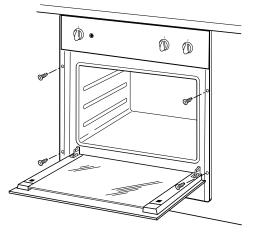
Ensure that the oven is fixed in a perfectly stable fashion, as shown, and that the electrical parts are isolated so that they do not come into contact with the metal parts. In addition, the adhesive that bonds the laminate to the unit must be resistant to temperatures of not below 90°C to avoid deformation and ungluing of the surface.
