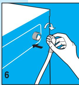
**N.B.** On electronic washing machines fitted with a dual solenoid valve (hot and cold water), connect the red hose to the hot water supply valve and the other hose to the cold water supply valve.
