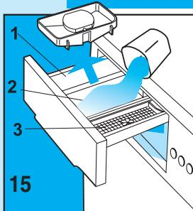
The washing machine has a three-compartment detergent drawer.
