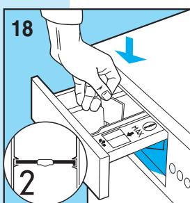
▼ Correctly insert the dividing wall in the guides (fig. 18)
