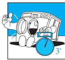
*The door can only be opened approximately three minutes after the end of each wash, as a safety device has been fitted to protect from accidental opening.*
