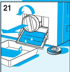
**ATTENTION!!** Before starting the operations described below, make sure that the washing machine is empty. Do not remove the filter while the machine is running, or when full of water.
