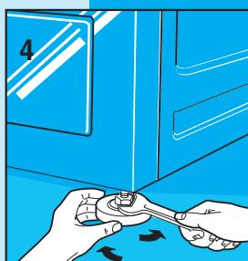
After selecting a suitable position, level the machine carefully using the adjustable feet (Fig. 4). Particular care must be taken when selecting the position, levelling the washing machine and ensuring the safety of lock nuts.
