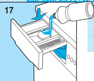
**N.B.** When using liquid detergent (recommended for programs without pre-wash), insert the special tray (if supplied) or the dividing wall inside the middle compartment "2" (as shown alongside), fig. 17/18, then pour the liquid detergent up to the maximum level indicated
