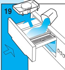
Remember to remove the liquid detergent tray or the dividing wall when using powder soap.
