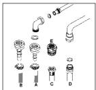
During the gas connection process, the pipe of the appliance should be kept stationary, while the connected part (mechanical, LPG or NG nut) is fixed. Always use the seals supplied in the spare set between the connection.
