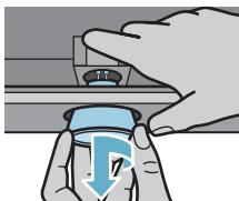
Only self-protection tungsten LED lamp, LED or self-protection metal halide lamp must be used.
