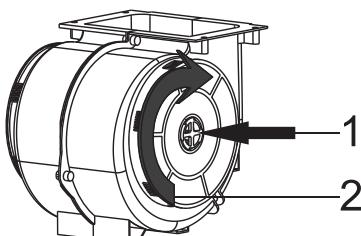
Slika 6: FILTER SA AKTIVNIM UGLJEM
