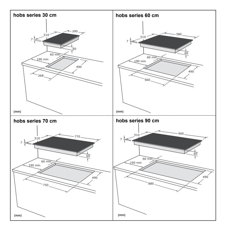
The appliance can be fitted into all types of units the walls of which resist an extra temperature of at least 65° C above the ambient temperature (EN 60335 - 2 - 6). Avoid installing it near inflammable materials, for example curtains, cloths etc.
