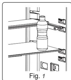
Adjustable glass shelf mechanism provides higher storage spaces with a simple movement.
