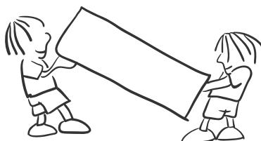
**Always carry your appliance in the upright position. If the appliance is carried in a horizontal position, it must be waited at least 3 hours before being switched on in order to prevent damage to its cooling system.**
