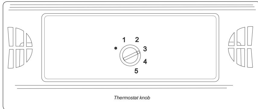
The thermostat automatically regulates the inside temperature of the refrigerator. By rotating the knob from position 1 to 5, colder temperatures can be obtained.
