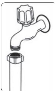
Do not use the water inlet hose of your old machine, if any. Use the new water inlet hose supplied with your machine instead. If you are going to connect a new or long-unused water inlet hose to your machine, run water through it for a while before making the connection. Connect the water inlet hose directly to the water inlet tap. The pressure supplied by the tap should be at a minimum of 0.03 Mpa and at a maximum of 1 Mpa.
