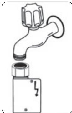
**NOTE:** Aquastop water spout is used in some models. In case of using Aquastop, a dangerous tension exists. Do not cut Aquastop water spout. Do not let it get folded or twisted.
