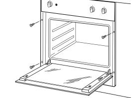
Ensure that the oven is fixed in a perfectly stable fashion, as shown, and that the electrical parts are isolated so that they do not come into contact with the metal parts. In addition, the adhesive that bonds the laminate to the unit must be resistant to temperatures of not below 90°C to avoid deformation and ungluing of the surface.
