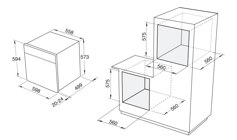
Put the oven into the recess laying it on the base and pushing it until the lateral jambs touch the sides of the unit.
