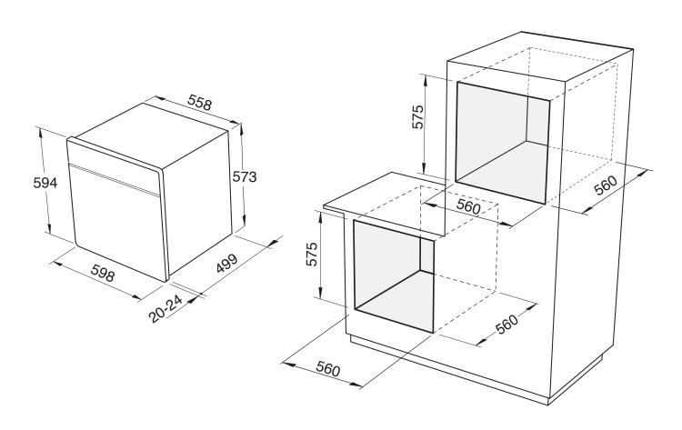
Put the oven into the recess laying it on the base and pushing it until the lateral jambs touch the sides of the unit.
