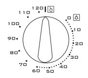
When the time that has been programmed has lapsed, the buzzer sounds and at the same time the oven is automatically switched off. To use the oven with the manual function, excluding the timer, put the knob back to its original position, rotating it in an anticlockwise direction by one notch until the reference of the knob coincides with the [b] symbol on the control panel.
