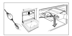
Place it on the support rack using the band on the bar which is near the handle. Put the drip tray on the lower shelf, remove the handle of the bar during cooking. The handle is only to make it easier to remove the food when it is cooked.
